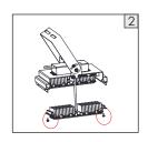
2. Undo the screws on ends of the module.
