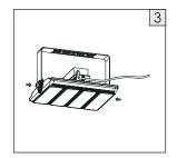
Loosen the screws on the sides. Adjust the body to a right angle. Tighten up the screws.
