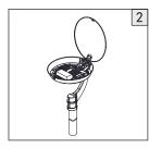
Undo the screws and connector for the module, and replace it with a new one. Tighten up again.
