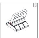
Loosen the screws on two sides of the bracket to adjust the fixture to a proper angle. Tighten up the screws.
