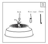
Mount the fixture with a hook, a wire rope or a chain through the hoisting ring, and tighten up.
