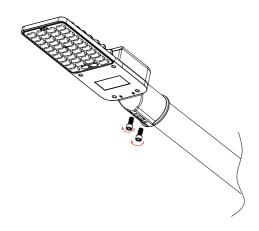
Loosen the the screws for fixture mounting. Stick the pole arm into the mounting tube. Fasten up the two screws evenly in a way of multiple interchange instead of one-by-one, making sure of the comliance of torque force. Installation finished.
