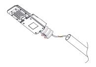
2. Loosen the monting screws on the pole sleeve.
