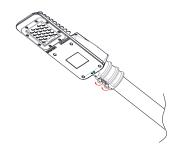
3. Mount the luminaire onto a pole. Tighten up the screws to fixate it.
