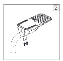
2. Loosen the screws on the tube. Mount the fixture onto the pole and tighten up the screws to fix it. Installation finished.
