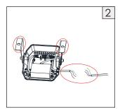
2. Connect the wires to AC input. Make sure it grounded sufficiently.
