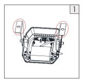
1. Mount the fixture with screws at the bracket. (Mounting screws are not provided in package. Screw hole diameter: Ø11mm.)
