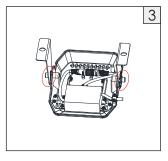
3. Loosen the screws on brackets to adjust to a proper angle.
