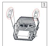
Fixate the luminaire onto the mounting surface with screws. (recommend M10 screws) .
