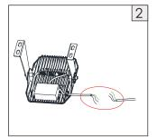
2. Connect the wires to AC input. Make sure it grounded sufficiently.
