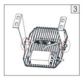
3. Loosen the M10 screws on brackets to adjust to a proper angle.
