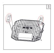
Fixate the luminaire onto the mounting surface with screws. (recommend M10 screws)
