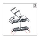
Undo the screws on ends of the module.
