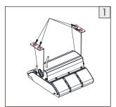
1. Fixate the luminaire onto the mounting surface with screws (recommend M10 screws)
