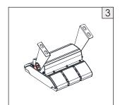
3. Loosen the M8 screws on brackets to adjust to a proper angle.
