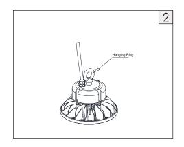
2. Hook and hang the luminaire to the ceiling. Installation finished.
